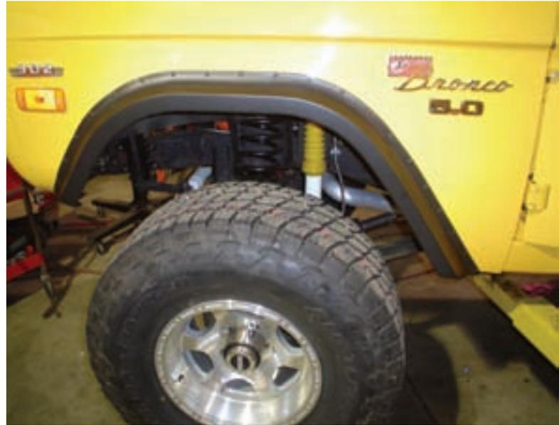
A 3" suspension lift from Superlift along with a 1" body lift made room for the 325/70-16 Nitto Terragraper's on 16x10 American Racing wheels. Trimming the front fender and mounting Bushwacker flares was also done to cover the larger tread and match the already existing rear flares. With this combination there were no clearance issues, rubbing problems or fitment concerns at all. And the Nitto tires balanced out perfectly and drive smooth and quiet on the highway.
