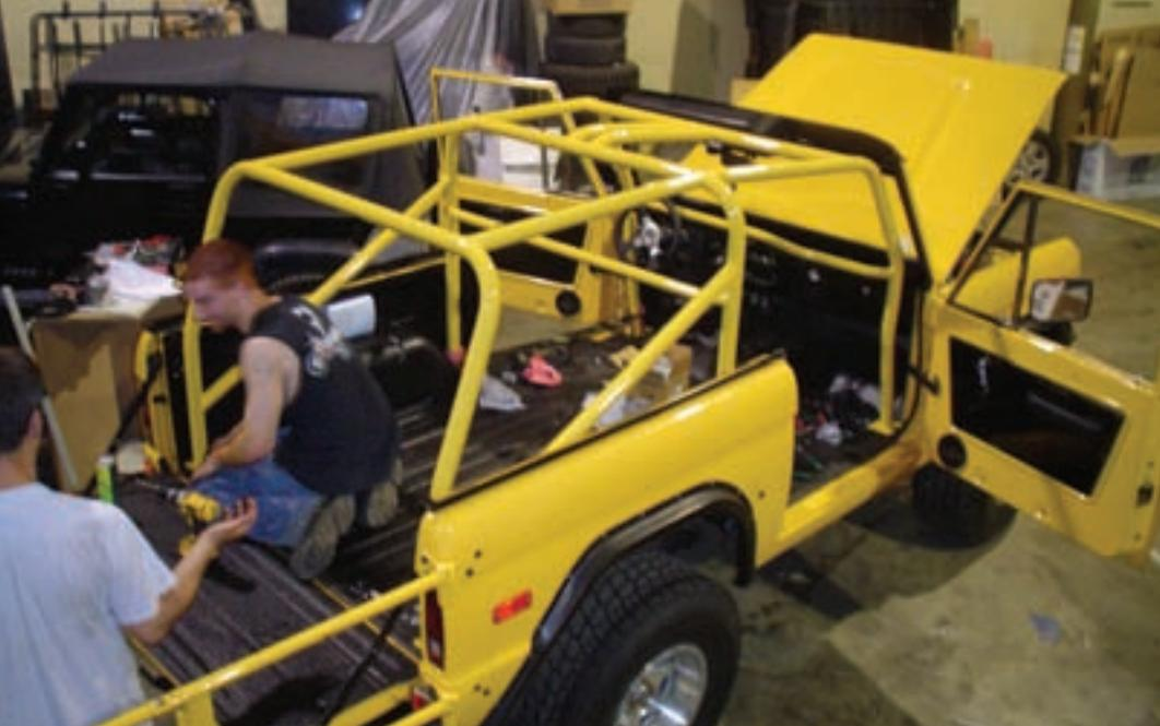
designed specifically for the early Bronco's and hold a Warn 9.5Ti winch in front and a built in tow hitch in the back. They even accommodated the 1" body lift by drilling extra holes in the mounting brackets.
